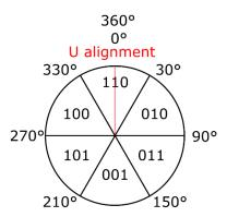
AZ3Plus50 can handle incremental encoder with Hall, with every displacement between U phase rising edge and zero mark. The displacement is configurable through *Encoder phase displacement*, for example if zero mark is positioned exactly on U phase rising edge, then *Encoder phase displacement* must be set to zero. In the following image is possible to understand how setting *Encoder phase displacement* in order to obtain the desired displacement.
