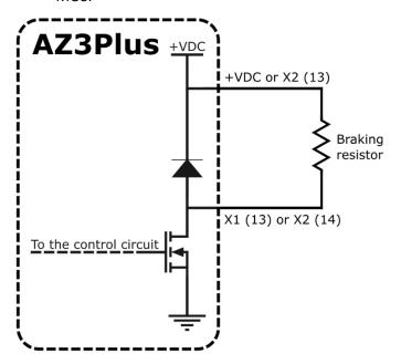
• The drive can manage an electromechanical brake without relay/contactor. The current of the electromechanical brake must not exceed 1.5 A.
