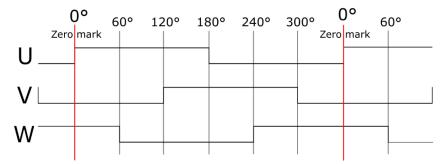
**EXAMPLE:** if a motor has an incremental encoder with Hall with a displacement between U phase rising edge and zero mark of 180° (3.14 rad), it is sufficient to set *Encoder phase displacement* to 3.14.
